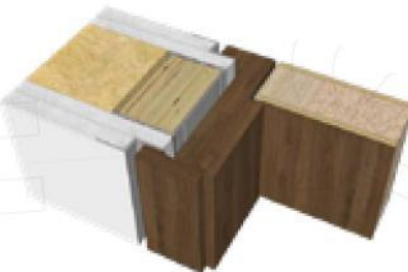
Drywall wall with shadow gap feature +Single rabbet jamb with 1 side adjustable casing
