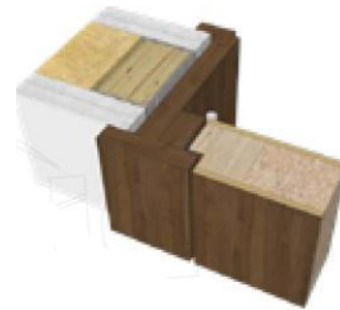
Drywall outside flush jamb with in-swing door
