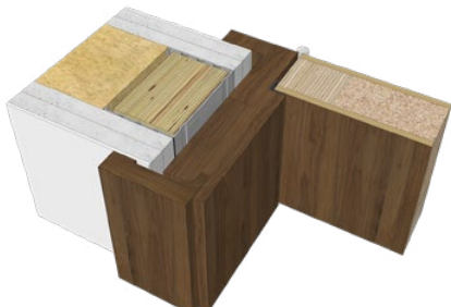
Drywall single rabbet jamb with 1 side adjustable casing
