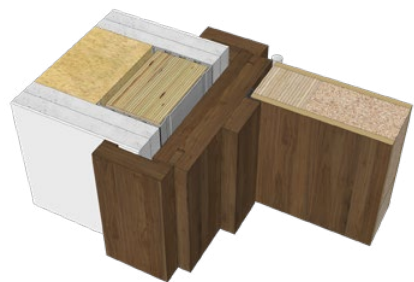
Drywall double rabbet jamb with 2 sides adjustable casings
