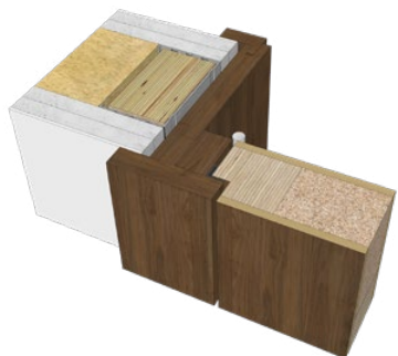
Drywall outside flush jamb with in-swing door
