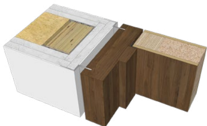
Drywall with shadow gap feature + Double rabbet jamb
