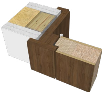
Drywall outside flush jamb with in-swing door
