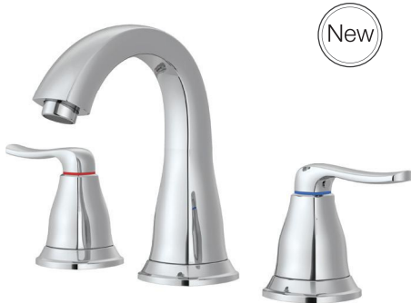
Pending Pa-1028-XX Two Handle Widespread Lavatory Faucet. Lead-free brass waterway, 1/2 Ceramic cartridge Zinc alloy Gravity casting spout, Zinc alloy handle Quick mounting nut, Quick connection hose 30" PEX inlet hose Plastic two piece pop-up waste Neoperl aerator: PCA 1.2GPM
