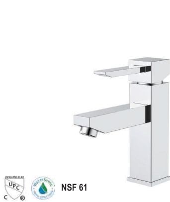
Ta-6781-XX One-Handle Bathroom Faucet 35mm Ceramic cartridge Brass body. Zamak lever handle Finishes : CP, BN, MB, ORB, PN, BG, BP
