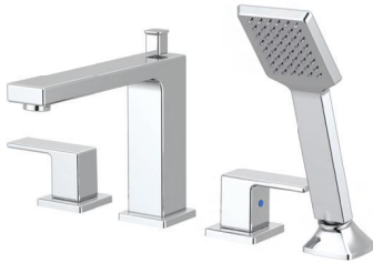
Ta-809S-xx Two Handle 4PC Roman Tub Faucet 35mm Ceramic cartridge. Brass body and spout Zamak lever handle. One function hand-shower Finishes : CP. BN. MB. ORB. PN
