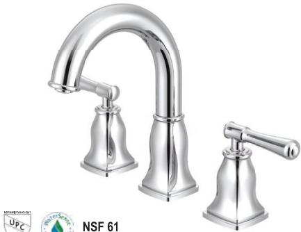
Ta8028-XX Two Handle Widespread Bathroom Faucet. 1/2 Ceramic cartridge. Brass spout and waterway. Zamak lever handle. Quick connecting T-hose Finishes : CP. BN. BP. BG. MB. ORB. PN
