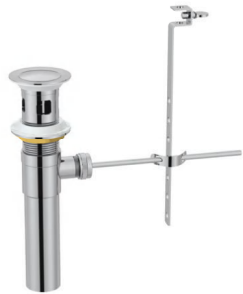
8622Q0703A0 Two Piece Pop-up Drain 1-1/4"x8" Brass body Stainless steel tube Adjustable lift rod and horizontal ball joint rod
