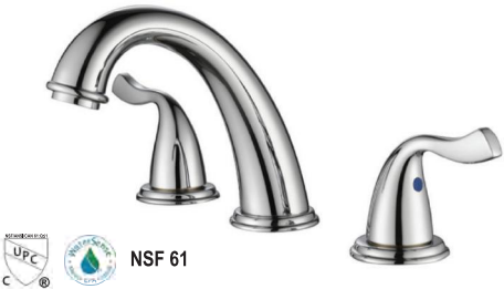
Ta-8298-XX Two Handle Widespread Lavatory Faucet. 1/2 Ceramic cartridge. Hybrid waterway Zamak lever handle and casting spout. Quick connection Finishes : CP. BN. MB. ORB. BG. BP. WP. PN
