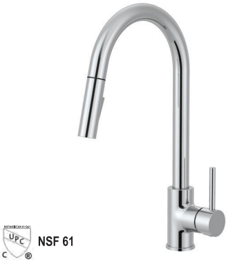
Ta629P-XX One-Handle High Arc Pulldown Kitchen Faucet 35mm Ceramic cartridge Zamak body and lever handle. Stainless steel spout Brass waterway. Two functions pull-down spray 1.5m quick connecting nylon braided hose Finishes : CP, BN, MB, ORB, PN, BG
