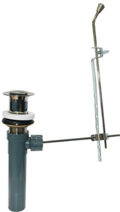
8635Q0591A0 Two Piece Pop-up Drain 1-1/4"x8" Stainless steel body Plastic tube Adjustable lift rod and horizontal ball joint rod
