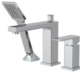
Ta-809R-XX One Handle 3PC Roman Tub Faucet 35mm Ceramic cartridge. Brass spout and waterway Zamak lever handle. One function hand-shower Finishes : CP. BN. MB. ORB. PN
