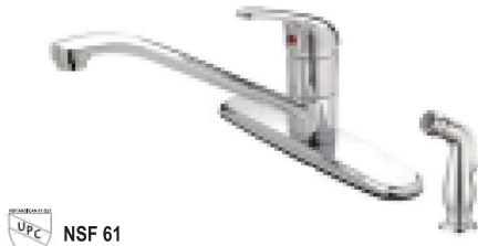
Ta-7653-XX One-Handle Kitchen Faucet with sprayer 35mm Ceramic cartridge Hybrid waterway. Zamak lever handle Brass spout. Stainless steel deckplate Finishes : CP. BN. MB. ORB. BP. WP
