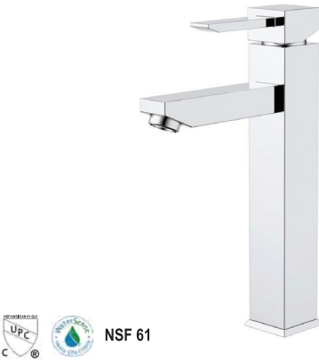
Ta-6780-XX One-Handle High Arc Bathroom Faucet 35mm Ceramic cartridge Brass body. Zamak lever handle Finishes : CP, BN, MB, ORB, PN, BG, BP
