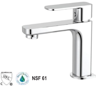
Ta8071-XX One-Handle Bathroom Faucet 35mm Ceramic cartridge Brass body. Zamak lever handle Finishes : CP, BN, BP, BG, MB, ORB, PN
