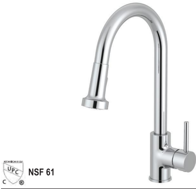
Ta-629P-1-XX One-Handle High Arc Pulldown Kitchen Faucet 35mm Ceramic cartridge Zamak body and lever handle. Stainless steel spout Brass waterway. Two functions pull-down spray 1.5m quick connecting nylon braided hose Finishes : CP, BN, MB, ORB, PN, BG
