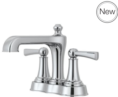
Pending Ta-D0002-XX Two Handle Centerset Bathroom Faucet. Hybrid waterway, 1/2 Ceramic cartridge Zinc alloy Gravity casting spout, Zinc alloy handle Stainless steel deckplate Plastic two piece pop-up waste Neoperl aerator: PCA 1.2GPM
