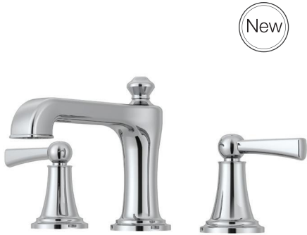
Pending Ta-D0008-XX Two Handle Widespread Lavatory Faucet. Lead-free brass waterway, 1/2 Ceramic cartridge Zinc alloy Gravity casting spout, Zinc alloy handle Quick mounting nut, Quick connection hose 30" PEX inlet hose, Plastic two piece pop-up waste Neoperl aerator: PCA 1.2GPM
