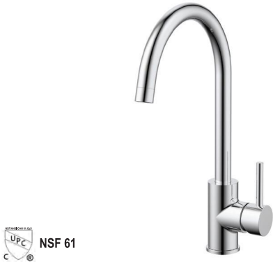
Ta-6293-XX Kitchen Faucet 35mm Ceramic cartridge Brass body and spout. Zamak lever handle Finishes : CP, BN, MB, ORB, PN, BG
