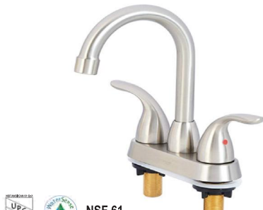
Ta-7652-XX Two Handle Centerset Bathroom Faucet. 1/2 Ceramic cartridge. Hybrid waterway Zamak lever handle and shell Finishes : CP. BN. BP. MB. ORB. WP. PN
