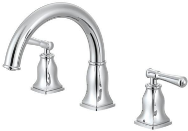
Ta802R1-XX Two Handle 3PC Roman Tub Faucet 1/2 Ceramic cartridge. Brass spout and waterway Zamak lever handle. Without hand-shower Finishes : CP. BN. MB. ORB. PN, BP
