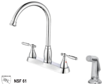
Ta-8293-XX Two-Handle High Arc Kitchen Faucet with sprayer 1/2 Ceramic cartridge. Hybrid waterway Zamak lever handle . Stainless steel spout and deckplate Finishes : CP. BN. MB. ORB. BP. WP
