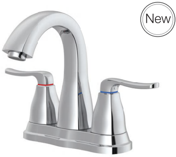
Pending Pa-1022-XX Two Handle Centerset Bathroom Faucet. Hybrid waterway, 1/2 Ceramic cartridge Zinc alloy Gravity casting spout, Zinc alloy handle Stainless steel deckplate Plastic two piece pop-up waste Neoperl aerator: PCA 1.2GPM
