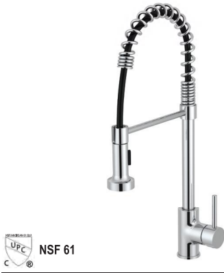
Ta629S-XX One-Handle Pull-Down Spring Kitchen Faucet 35mm Ceramic cartridge Zamak body and lever handle. Stainless steel spring Brass waterway. Two functions pull-down spray. 1.5m quick connecting nylon braided hose Finishes : CP, BN, MB, ORB, PN, BG
