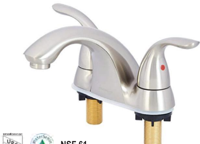
Ta-7652-XX Two Handle Centerset Bathroom Faucet. 1/2 Ceramic cartridge. Hybrid waterway. Zamak lever handleStainless steel spout and deckplate Finishes : CP. BN. MB. ORB. BP. WP. PN
